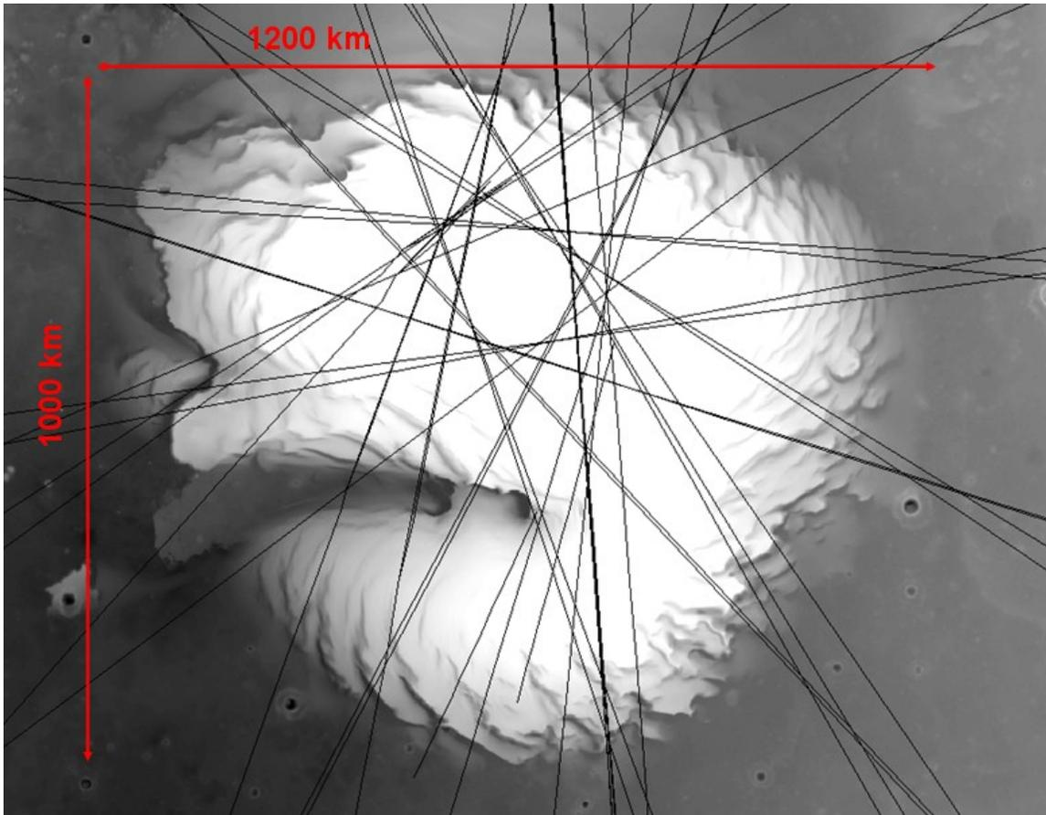
*Figure 2: MOLA Topography data of the Mars North Pole with the 31 selected footprints projected on it.*
